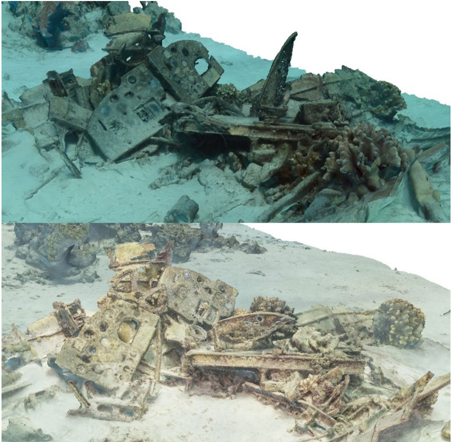
Fig. 24 Demonstrating changes on site between 2017 (top) and 2023 (bottom). Note the cockpit panel has been disarticulated and incorrectly reconstructed between dates
