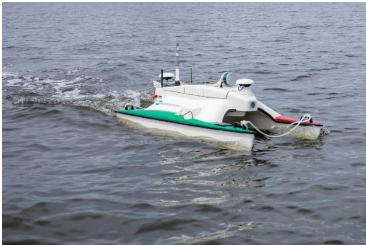
Figure 7: SR-Surveyor M1.8 autonomous surface vehicle used for the acoustic surveys.
