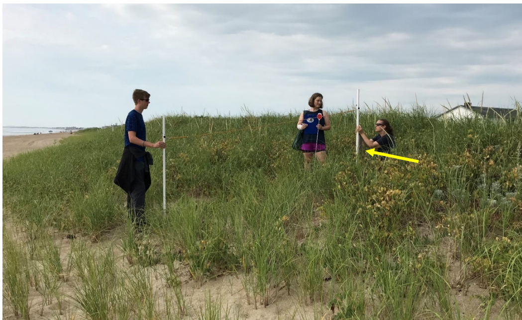
Figure 2-8: First measurement at a dune station starting from the wooden stake in the foredune ridge. The stake is low enough for the profilers to see over the top, but high enough that it does not become buried in sand deposited in the dunes. The profile rod is placed against the wooden stake (arrow) by the landward profiler.
