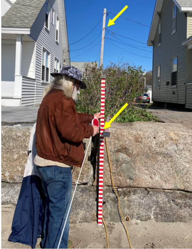
Figure 2-2: Example of aligning a station marker and a “back site” point of reference at a seawall station. Left: the bottom arrow points to the station marker (black dot on wall) and the top arrow points to the back reference site (telephone pole). Right: the corresponding shore-normal transect down the beach resulting from the alignment of these two reference points. Note the reflector stake placed at the station marker for better visibility.
