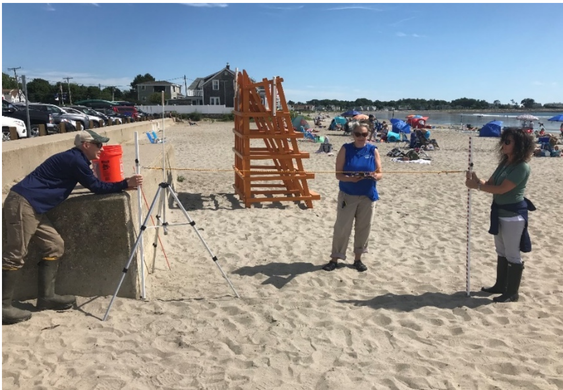
Figure 2-14: The first measurement or "jump" of a profile, where the landward rod begins at the station marker. Both rods are perpendicular to the sand surface and the rope in between is pulled taut. In this case, the slope of the beach is downward, and therefore the elevation measurement will be negative.
