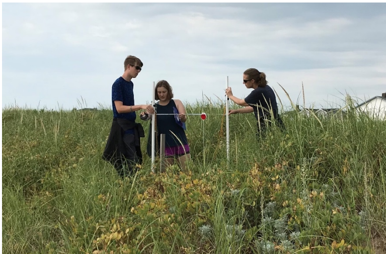
Figure 2-19: An example of how to measure a short jump. A measuring tape is used here to measure the distance between the profile rods.
