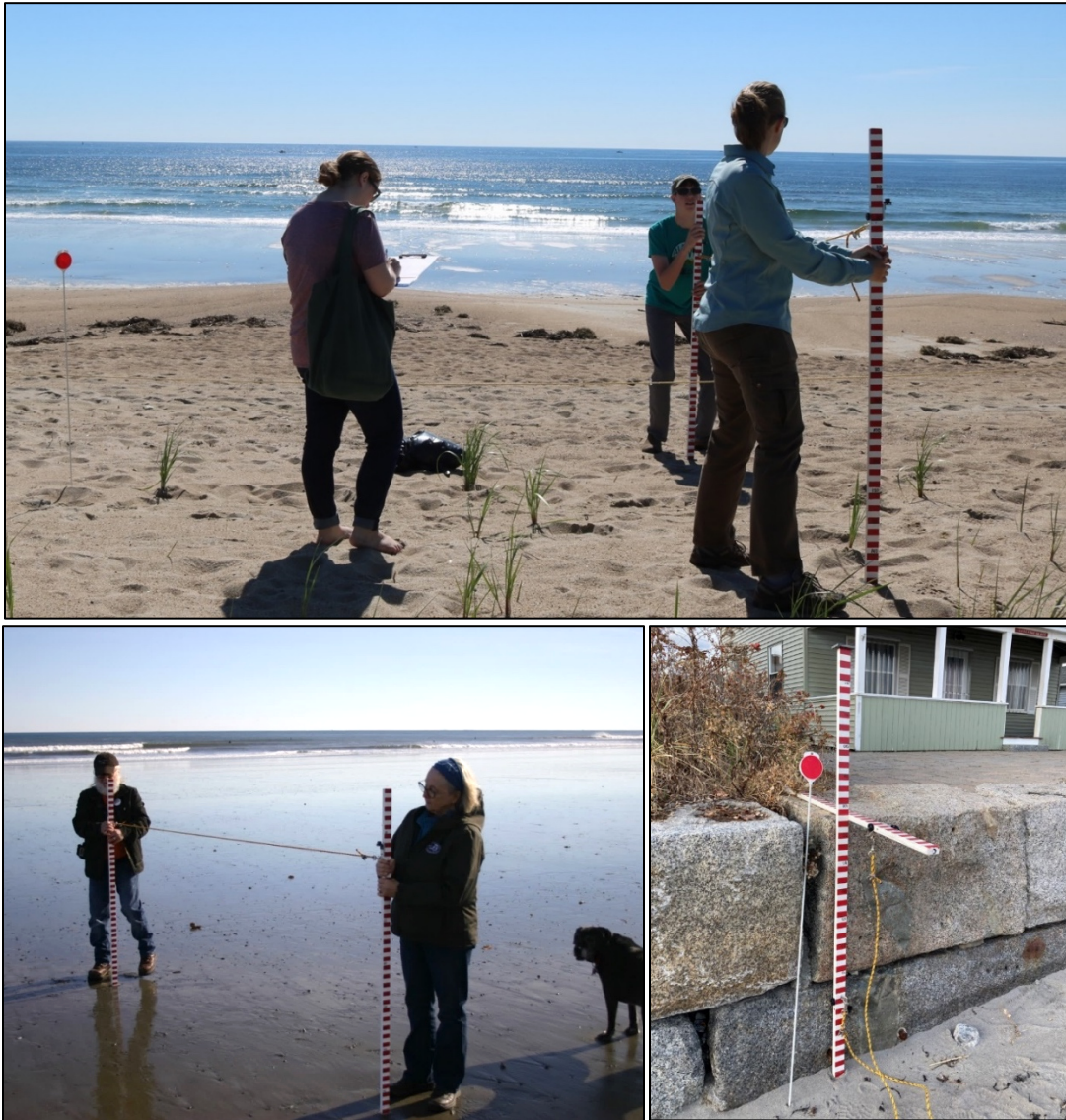
Figure 2-1: Beach profiling using the Emery method at Seabrook Beach (upper) and Jenness Beach (lower), NH in 2018.
