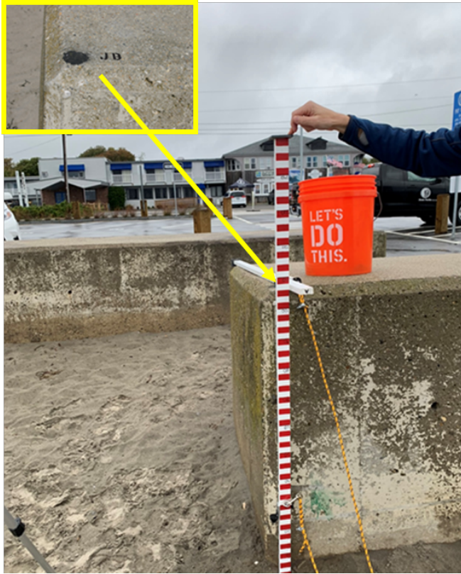
Figure 2-12: Photograph showing how to measure the distance from the station marker to the beach surface. The inset shows the mark on the seawall indicating the station marker location. The rod is placed upside-down to measure the distance from the sand surface. The second rod is being used to create a flat surface on top of the seawall for an accurate measurement.
