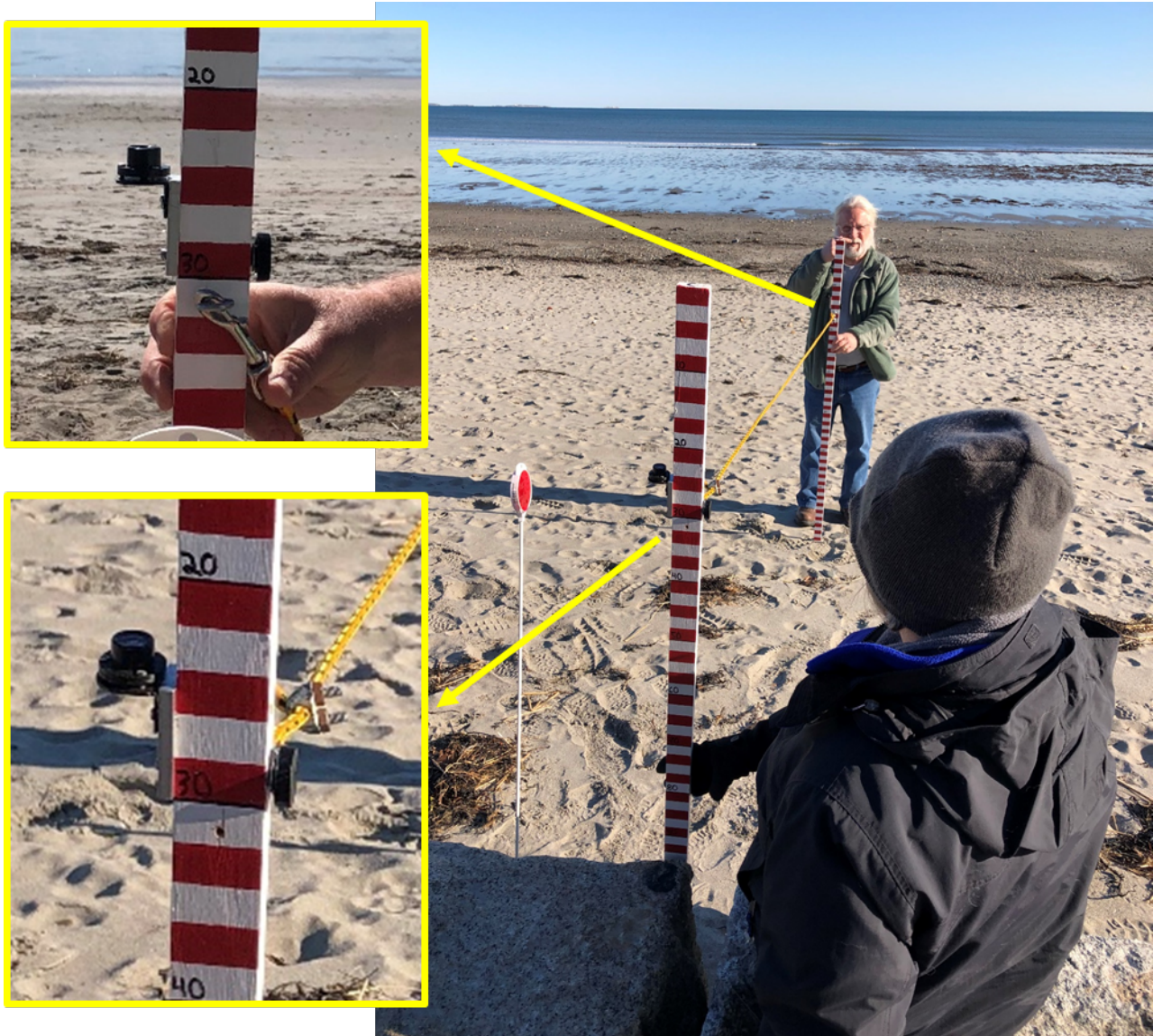
Figure A-2: Volunteers profiling with a completed profile rod set. The front side of each rod is painted with 2-centimeter increments and is connected by an approximately three-meter-long cord. Both rods have bubble levels. The cord is screwed onto the back of the landward rod (lower left-hand inset figure) and the front of the seaward rod (upper right-hand inset figure).
