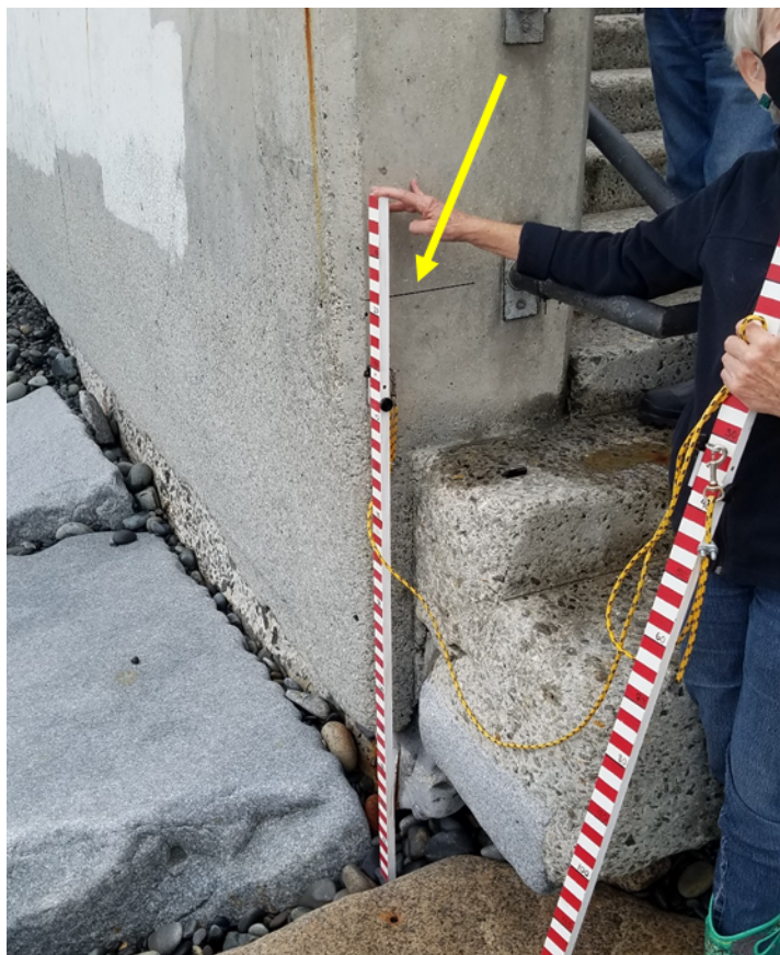
Figure 2-7: To facilitate measurements at a station where the sand surface height changes significantly (and becomes too low to measure with a single profiling rod), the NH VBMP has added a 1-meter mark on the seawall (arrow). The volunteers measure only from this line down to the sand.
