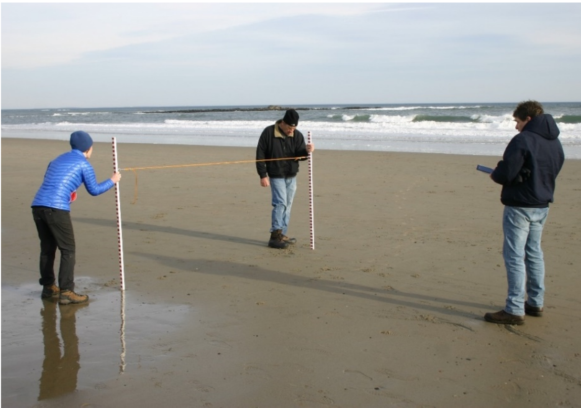
Figure 2-10: Volunteers profiling using the Emery method. Note that profile rods are vertical, and the rope is pulled taut.
