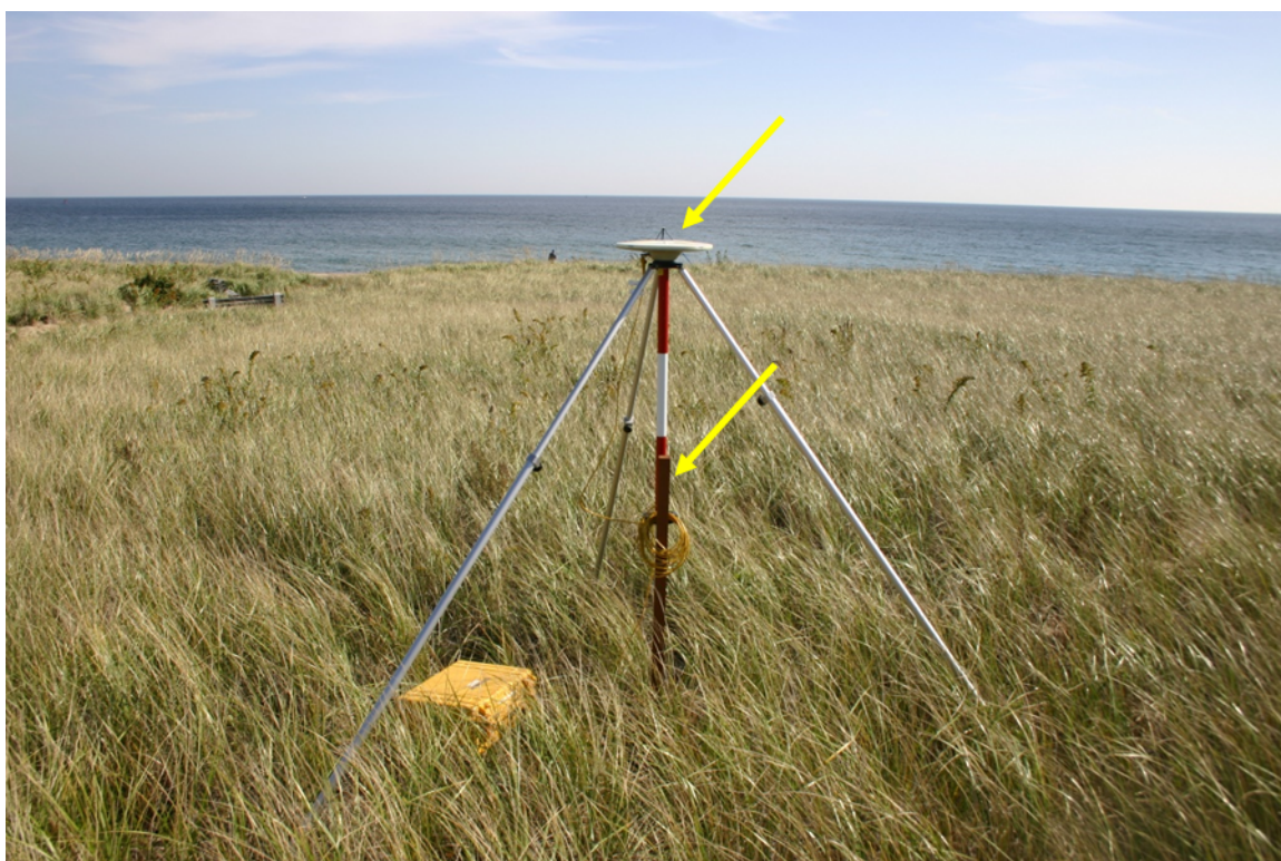
Figure 2-9: Leveling of a dune stake station marker (bottom arrow points to the wooden stake in the dunes) using GNSS antenna and receiver systems (top arrow).
