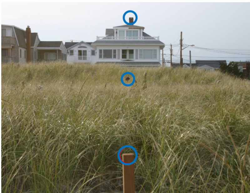
Figure 2-3: Example of aligning a station marker and a “back site” point of reference at a dune station, where the lower two circles mark the two dune wooden stakes (station marker and reference stake), and the upper circle marks an additional back site (chimney on house behind dunes).
