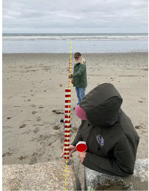
Figure 2-2: Example of aligning a station marker and a “back site” point of reference at a seawall station. Left: the bottom arrow points to the station marker (black dot on wall) and the top arrow points to the back reference site (telephone pole). Right: the corresponding shore-normal transect down the beach resulting from the alignment of these two reference points. Note the reflector stake placed at the station marker for better visibility.
