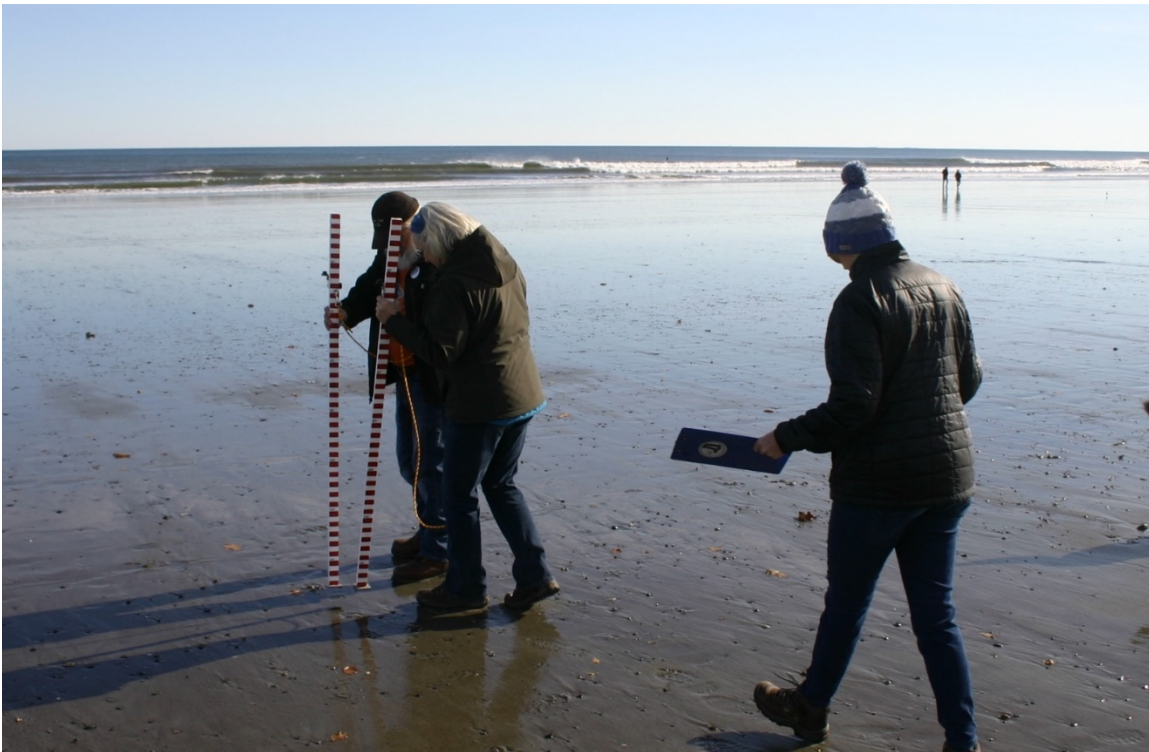
Figure 2-16: Continuing to another “jump.” The landward profiler places their profiling rod in the same footprint as the seaward rod before the seaward profiler continues down the beach to align the profile rod for the next “jump” along the transect.
