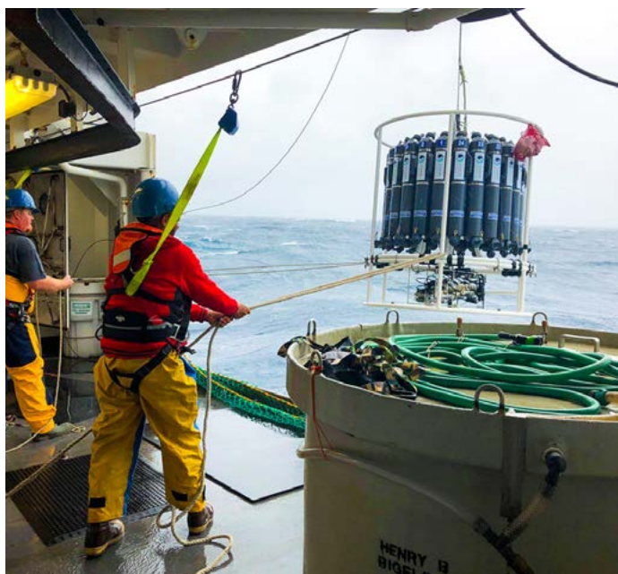
Crew deploy an ocean chemistry sensing array on the second East Coast Ocean Acidification research mission (ECOA-2)
