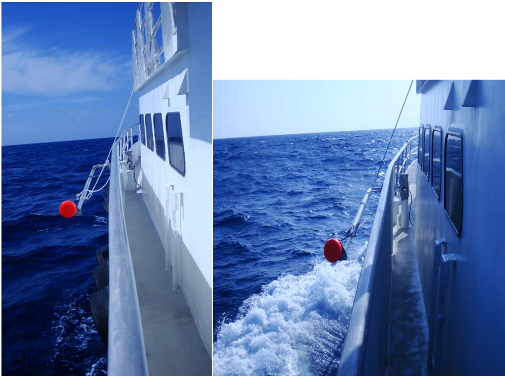
Figure 5. Transducer and pole on the M/V Spree
