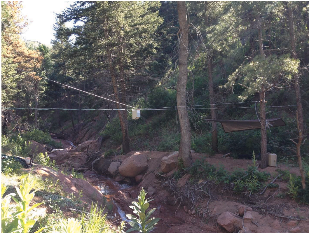
Fig. 3. Image of the deployment of the Lower Waldo radar streamgage, Waldo Canyon near Colorado Springs, Colorado. Photo credit: John Fulton/U.S. Geological Survey.
