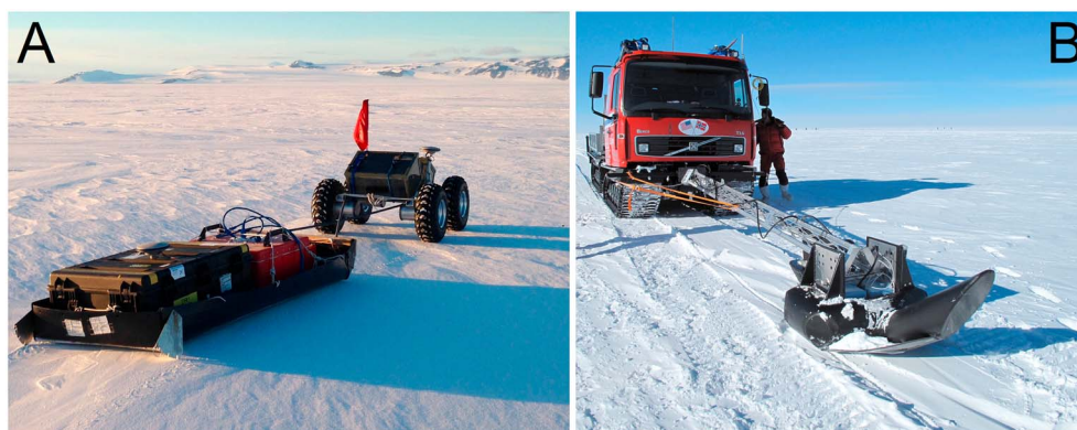
Figure 19. (a) An autonomous ground-penetrating radar unit (Yeti) being used to map near-surface buried crevasses at White Island, Antarctica, in October 2014. (Photo: Jim Lever) (b) High-frequency ground-penetrating radar pushed by a vehicle on the Norway-USA Scientific Traverse of East Antarctica during the International Polar Year, in November 2008. (Photo: Ted Scambos).
