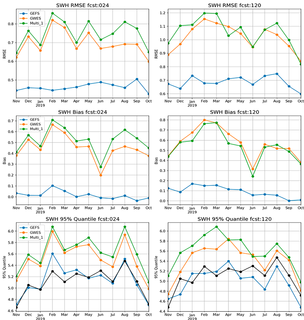
FIG. 3. Monthly SWH ( H_s ) validation statistics over the 1-yr evaluation period: (top) RMSE, (middle) bias, and (bottom) 95% quantile for the GEFSv12-Wave system (blue), the GWES system (orange), and the deterministic Multi-1 system (green). All values are in meters. Observed 95% percentile H_s are represented in black. Validation relative to altimeter data for November 2018–October 2019.
