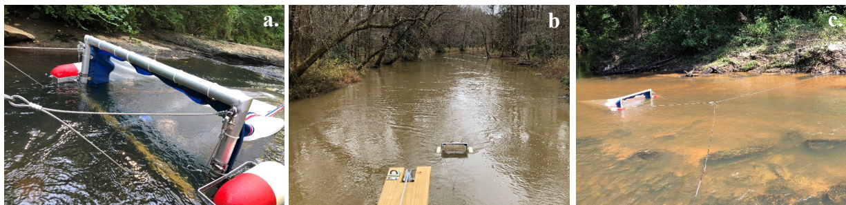
Figure 2. Sample trawl net with floats and velocity meter attached (a), sampling from a bridge (b), and sampling using cable suspended across the stream channel (c).
