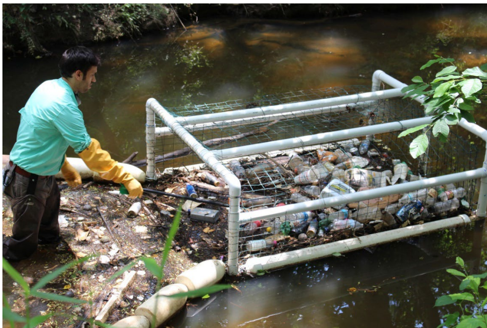
Figure 4. Removal of trash from the Litter Gitter© prototype following a storm event at Marsh Creek
