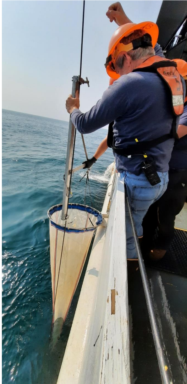
Figure 4. Deployment of 70-cm ring net from the side sample station of the NOAA Ship Henry B. Bigelow .
