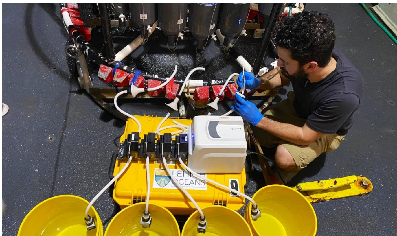
Alt Text: A researcher on deck carefully processing seawater samples using tubing, filters, and collection buckets, accompanied by specialized portable laboratory equipment labeled 'Lehigh Oceans'
