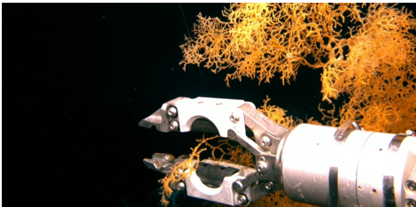
Alt Text: A remotely operated underwater vehicle's robotic manipulator arm carefully collecting samples of bright yellow-orange deep-sea coral against a dark ocean backdrop.
