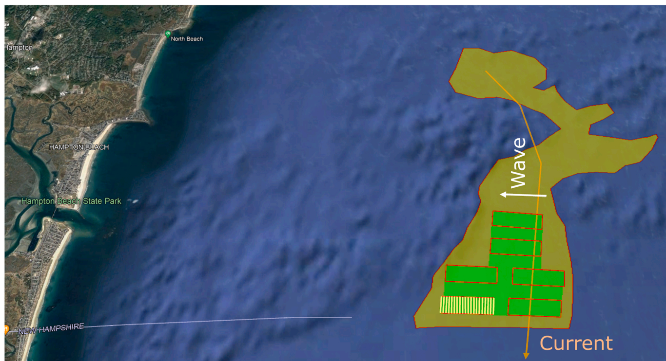
Fig. 6. Selected location and design of a 1009 acre mussel farm with plot outlines, average wave, and current directions. Each plot (red rectangles) has a dimension of 360 m x 1100 m. 1000 ft navigation is provided between plots. Mussel lines (Yellow) are 190 ft apart and 6 plots of 100 Acres with 6 x 20 (120) mussel lines. The orange arrow represents the mean current direction, and the white arrow represents the mean wave direction.
