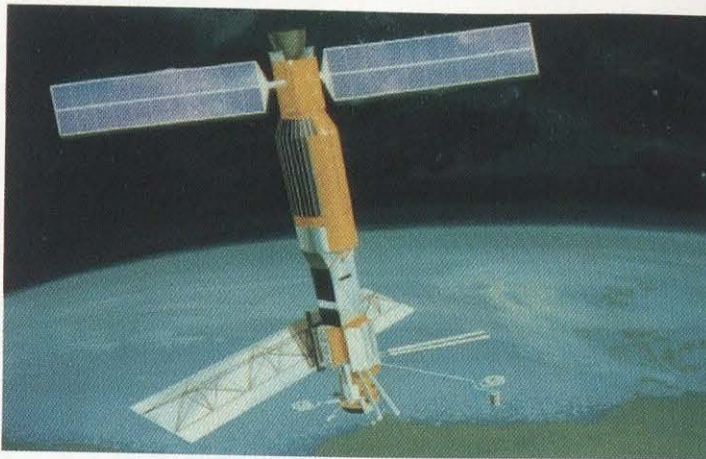
Figure 3-1. The Seasat satellite, launched in 1978, carried the first civilian synthetic aperture radar into space. (Photo: NASA)
