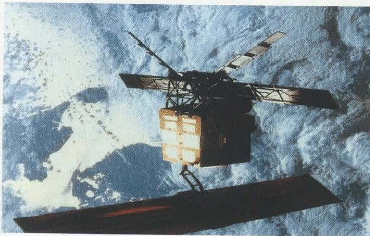
Figure 3-3. The European Space Agency ERS-1 satellite, launched in 1991, carries a C-band synthetic aperture radar for Earth and ocean observations. (Photo: European Space Agency)
