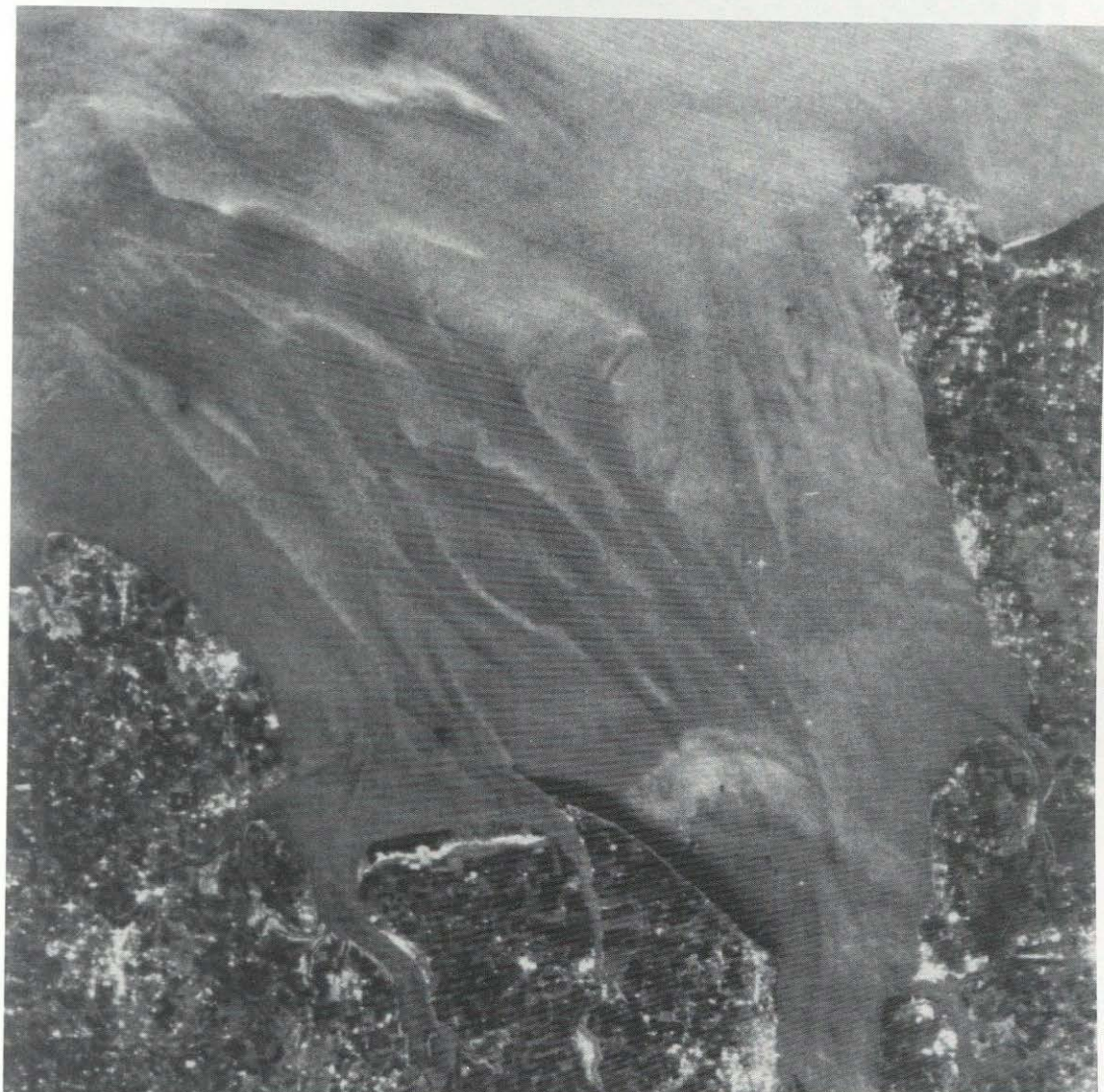
Figure 10-32. An ERS-1 SAR image of the English Channel north of the Thames River. Surface structure observed in the Channel is related to the seabed topography. Such imagery can aid in monitoring changes in shoals and sandbars, as well as providing input to littoral models supporting military expeditionary warfare operations. (Photo: European Space Agency and the Defence Research Agency-Farnborough)
