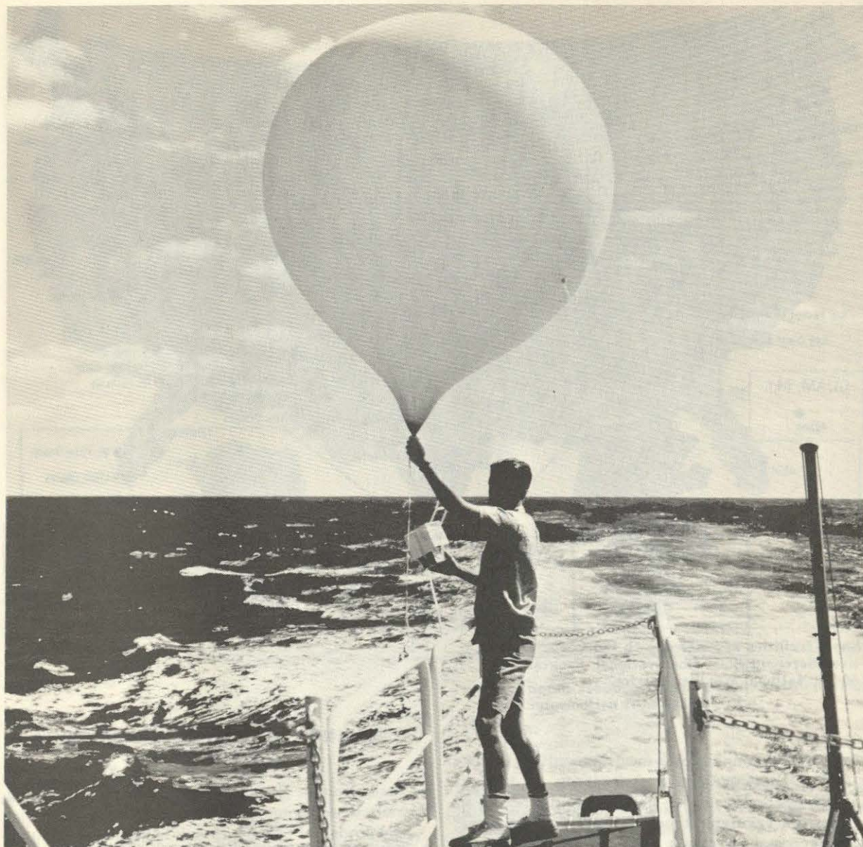
Release of radiosonde at sea to obtain upper air measurements. (National Weather Service)
