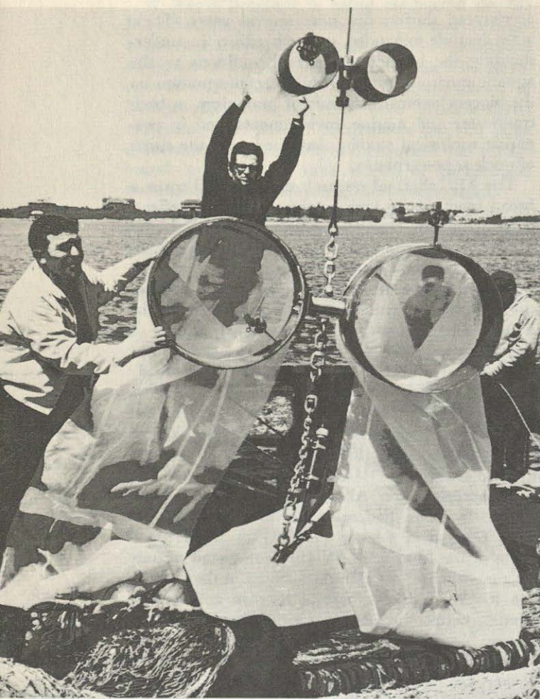
Double plankton-sampling array used to collect fish eggs and larvae to determine the distribution and abundance of living marine resources. (National Marine Fisheries Service)
