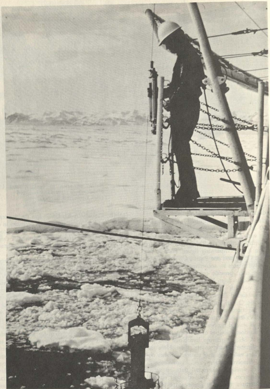
Salinity-temperature-depth (STD) system being lowered through the ice from U.S. Coast Guard Cutter Westwind .
