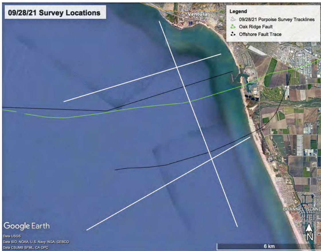
Map of CSEM survey lines collected on 09/28/21. The survey was designed to test the influence of faulting on the coastal aquifer supplying freshwater to the communities of Ventura and Oxnard.
