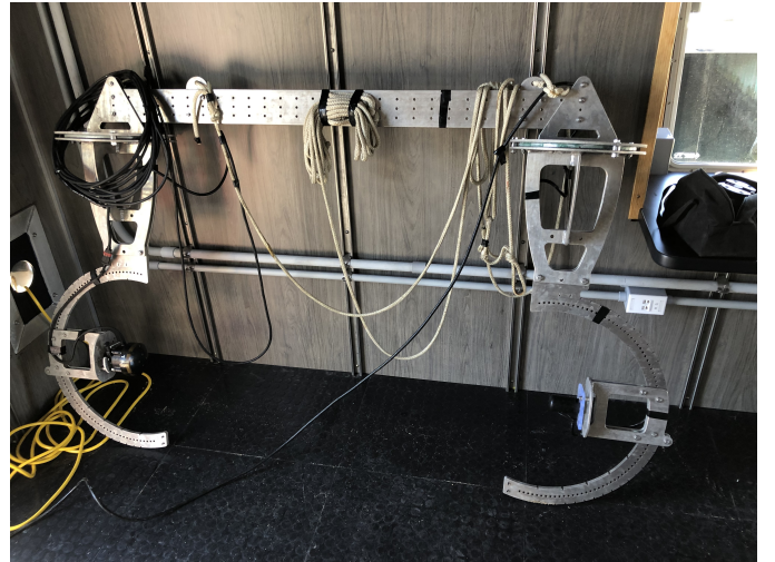
Fig. 6. Photo of dock test angle calibration rig, with iUSBL receiver on left, reference transducer on right, with both azimuth and elevation angle adjustment jigs. The device will be motorized to permit in situ scanning across azimuth and elevation.
