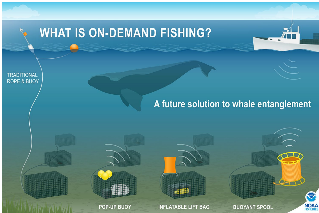
Figure 3. Example of the styles of on-demand gear designs currently available.
