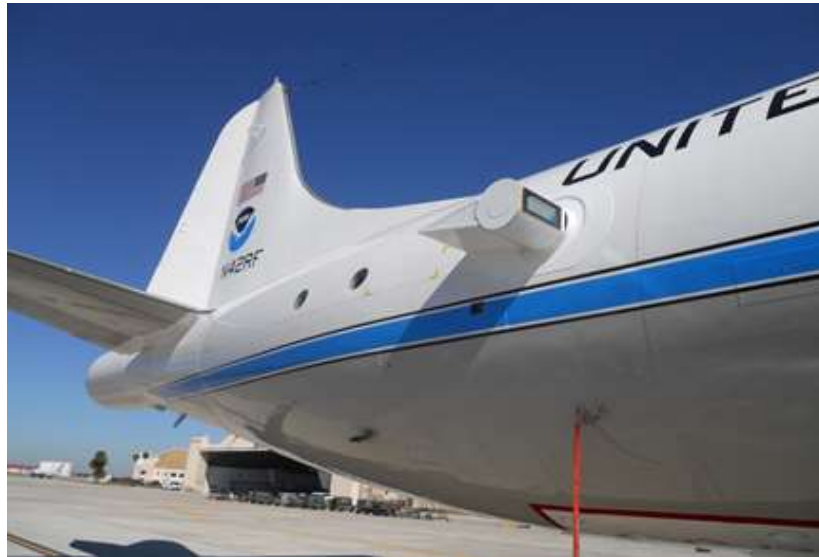
Figure 3. DWL scanner mounted on NOAA's P3 Hurricane Hunter reconnaissance aircraft. The side-mounted scanner permits observations below, at, and above flight level.
