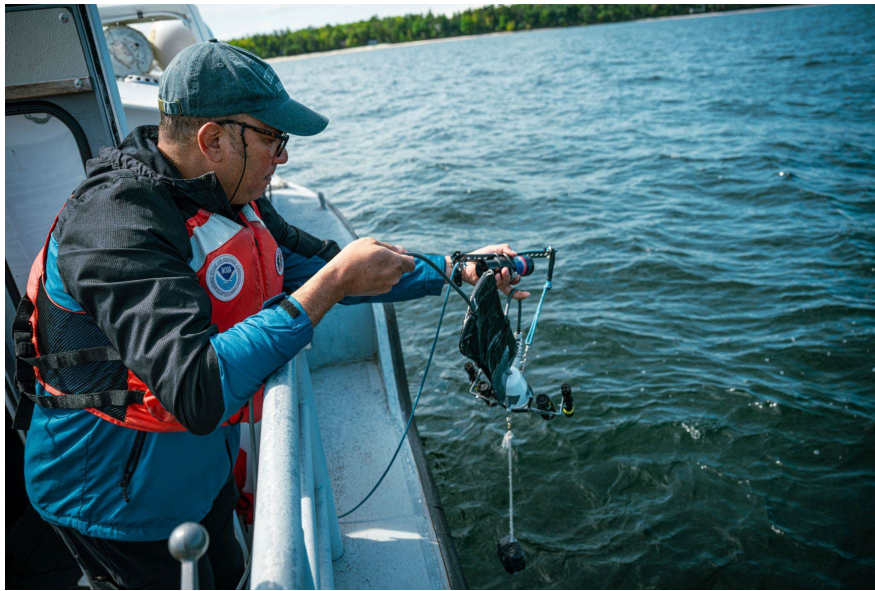
Figure 7. NCCOS staff deploying the Seaviewer drop camera off the vessel starboard. Credit: K. Staley/ MTU
