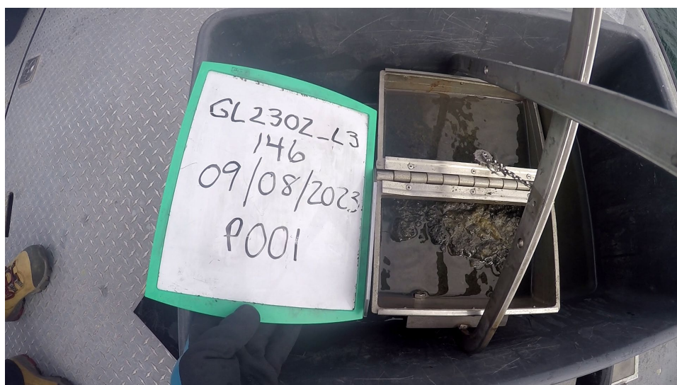
Figure 9. Standard Ponar dredge with the window opened, capturing a sandy sediment and a placard with the site information. Credit: A. Mabrouk/CSS, under contract to NOAA.
