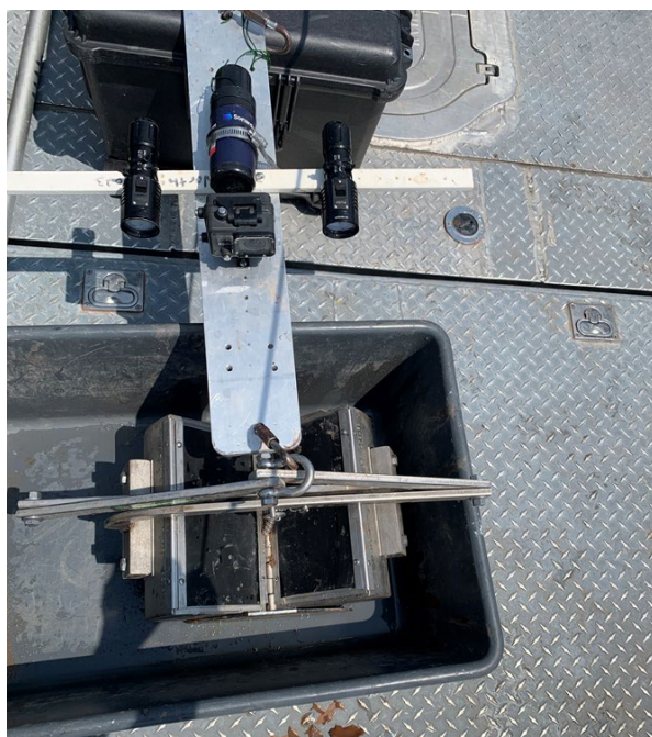
Figure 8. Ponar dredge with attached ultra-short baseline transponder, camera, and lights. Credit: A. Mabrouk/CSS, under contract to NOAA.
