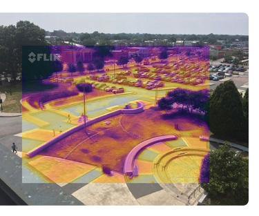
Specific data can also be collected for the project. The inset image, taken with a forward looking infrared (FLIR) camera, shows heat and is overlain on a regular photograph for context. In the FLIR image, lighter or brighter colors indicate warmer areas, while darker areas are cooler. Source: Science Museum of Virginia
