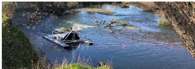
Figure 8. A Rotary Screw Trap in Reach 1 of the Restoration Area that is used to capture juvenile Chinook salmon for population estimates as they migrate downstream in the San Joaquin River. Photo credit: U.S. Bureau of Reclamation.
