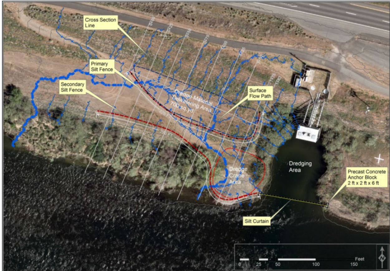
Figure 1. Location of Lewiston Water Intake structure and inlet channel proposed for dredging with measures to reduce sediment delivery to the Clearwater River.
