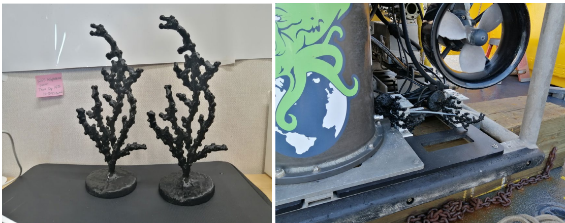
Figure 2.8. Polylactic acid 3D printed corals for testing (left); mounted to ROV for dives (right).
