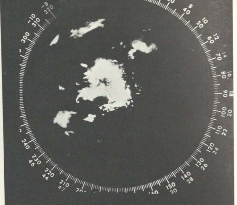
Figure 1.—PPI presentation of a squall line with hook-shaped echoes associated with tornadoes.
