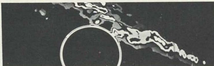
Figure 9.—PPI presentation of a squall line with VIP echo intensity contouring.
