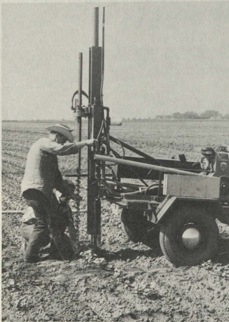
Portable drill sets access tubes for annual survey of soil moisture available to crops at start of growing season. Weather service contributes to this joint Federal, State, and local program of planning irrigation for efficient crop production and water use.
