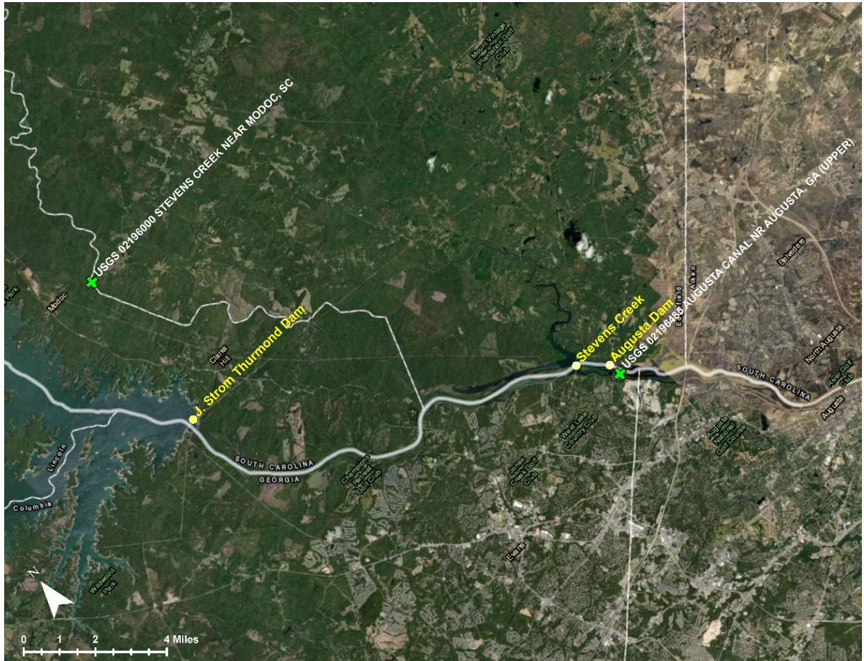
Figure 12. Map of Savannah River at Augusta Diversion Dam, showing USGS gage 02196000 in Stevens Creek near Modoc, SC and USGS gage 02196485 Augusta Canal near Augusta, GA.
