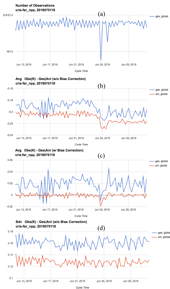
Fig. 19. The effects of the SNPP CrIS side switch on the (a) number of assimilated observations and on the mean departure between observed SNPP CrIS Side-2 brightness temperatures and simulated brightness temperatures from the six-hour forecast, or “guess”, (blue-line) and the analysis fields (red-line) through the side transition (b) before and (c) after bias correction at channel 91 ( 706.25 \text{ cm}^{-1} ) in the NOAA/NCEP operational data assimilation system. The standard deviation of the departures before bias correction is shown in (d).
