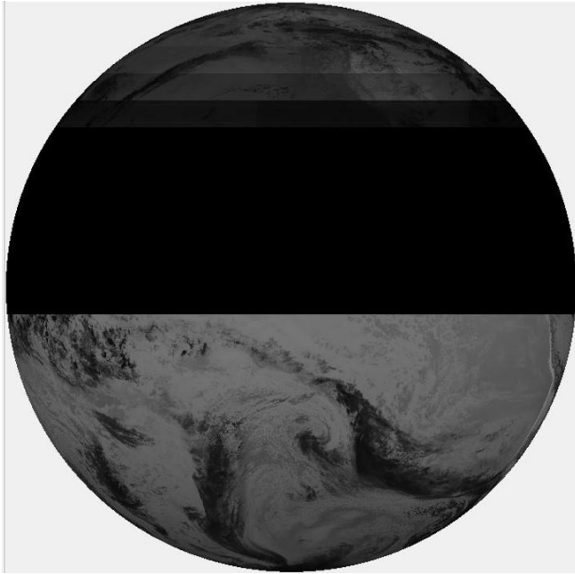
Fig. 4. A GOES-17 ABI L1b Full Disk image from July 18, 2019 at 1900 UT produced on the test processing environment showing what happens in the processing when the Predictive Calibration algorithm is active during a gain set switch. The applied detector gain extrapolation divergence continues until the ICT look that occurs halfway through the Full Disk. At that point the two ICT gain calibrations used for the extrapolation are utilizing the same gain set information.
