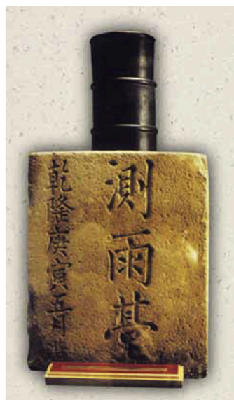
Fig. 26. Chukwooki, the traditional Korean rain gauge used to measure rainfall in major cities in Korea since 1441.
