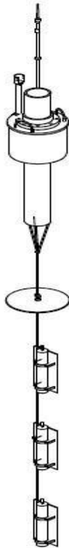
Figure 2. -- A drawing of the FSVPAD assembled for deployment (lines not to scale). The spar buoy contains batteries, a GPS, and communications electronics. A heave plate and the three hydrophones mounted on strongbacks are suspended below the drifter.
