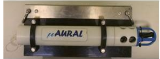
Figure 11. -- (Top) A drawing of the strongback assembly without hardware or a hydrophone. (Bottom) A strongback equipped with a hydrophone. When deployed the strongback should be oriented with the hydrophone towards the surface.
