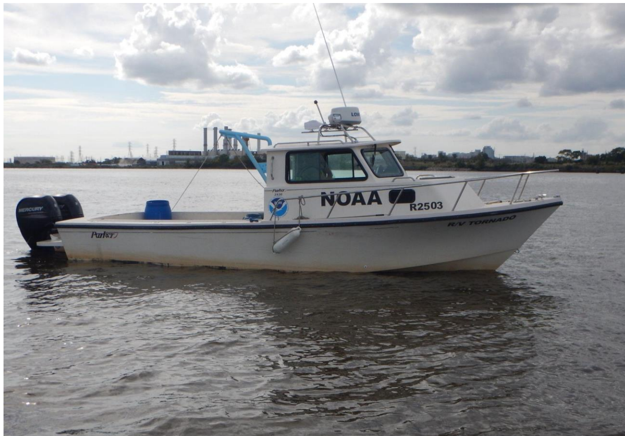
Figure 3. The NOAA research vessel (R/V) Tornado (25' Parker) equipped with a davit used for operations in the Charleston Harbor Reconnaissance.
