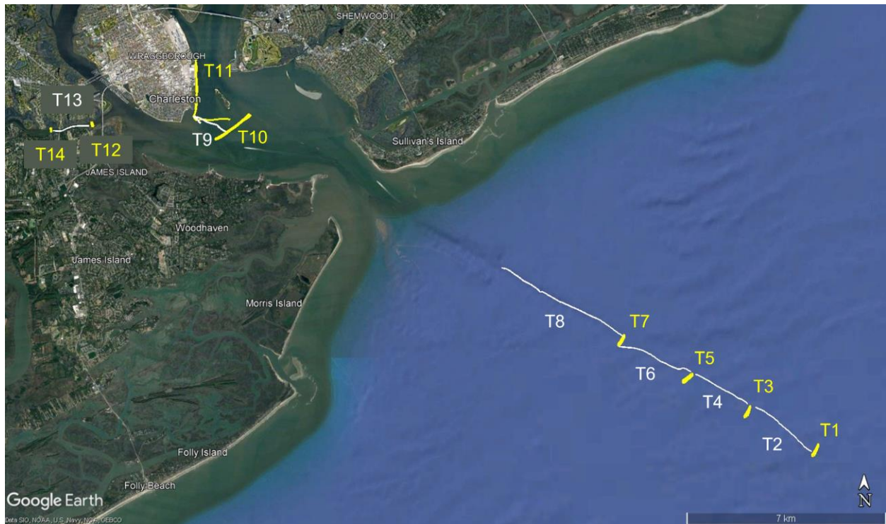
Figure 5. Nortek vessel-mounted (VM) system transect lines (T1-T14) outside and inside of Charleston Harbor and in Wappoo Creek. The white lines (T2, T4, T6, T8, T9, and T13) indicate 1 pass along the transect was completed. The yellow lines (T1, T3, T5, T7, T10, T11, T12, and T14) indicate transects along which multiple passes (4-17) were completed.
