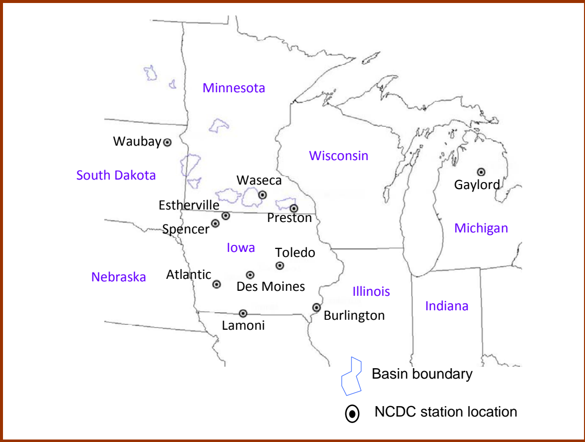
Figure 5. Locations of the eleven NCDC stations in the upper Midwest of the U.S. used for point-type soil temperature tests. The locations of the eight test basins are also shown.
