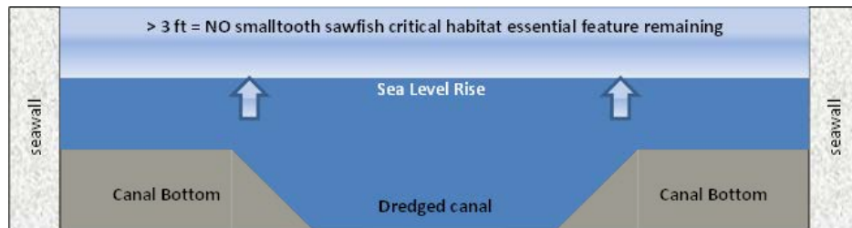
Figure 6. Diagram A depicts a cross section of a historically dredged channel/canal within the boundaries of the critical habitat units that has not been maintained. Diagram B depicts the typical cross section of a maintenance-dredged channel/canal. Diagram C
