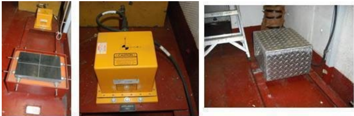
Figure 2. IMU and granite block (left), IMU (center), IMU under protective housing (right). All photos in the fan room.
