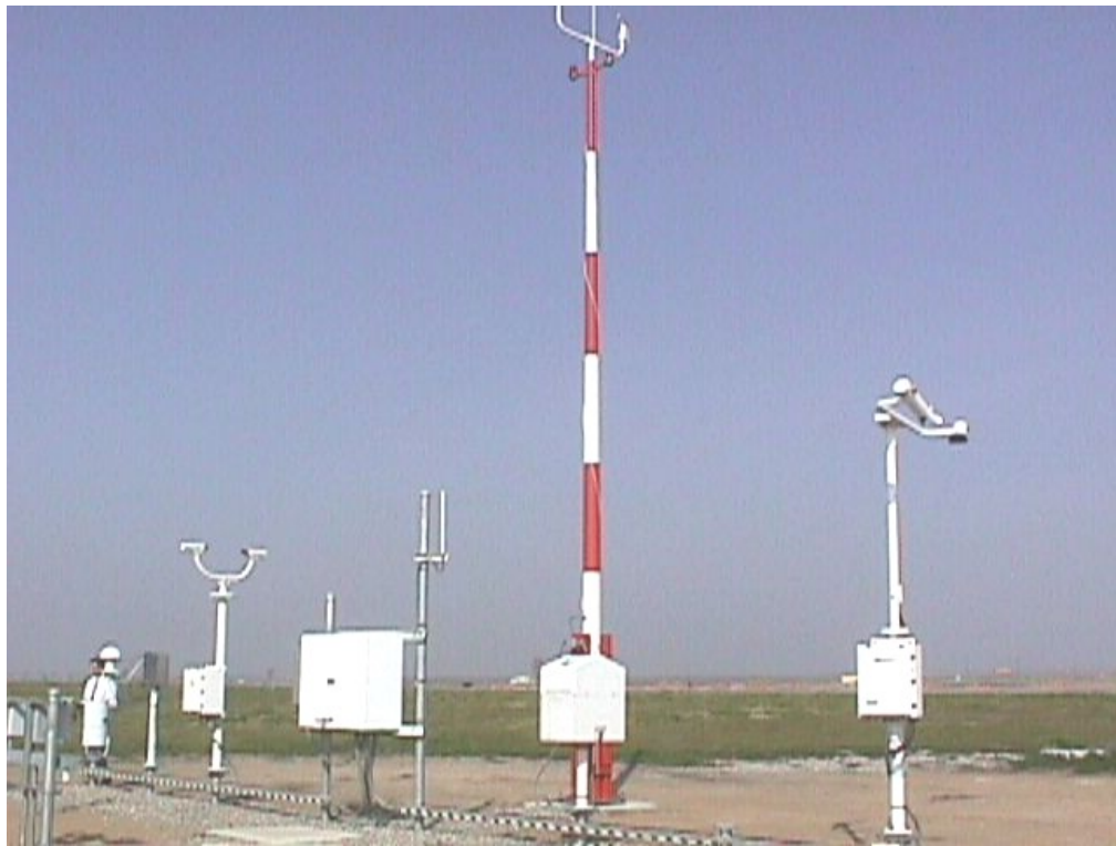
Figure 10 – The ASOS at Meadows Field in Bakersfield (Photo courtesy NWS Hanford Electronics Technicians staff).
