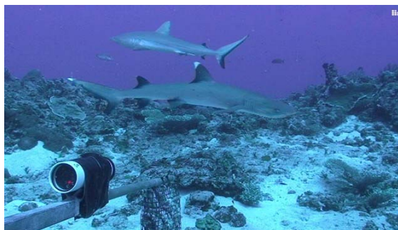
A) Figure A.4.1a--A) Stereo-baited remote underwater stereo-video system (Stereo-BRUVS). B) Frame grab from video footage collected (right camera). Note synchronising diode and bait bag in view.
