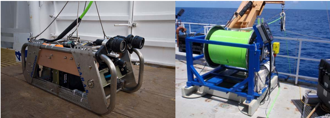
Figure A.3.2.1.--TOAD camera sled and remote-controlled winch.
