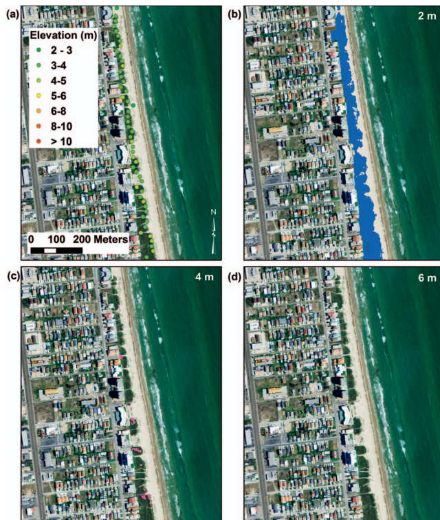
Figure 8. Example of area in developed segment with retaining wall of southern Padre Island showing (a) maximum dune crest elevations and areas of threshold elevations greater than (b) 2 m, (c) 4 m, and (d) 6 m NAVD88. Note there are no areas greater than 6 m in the beach and dune system.
