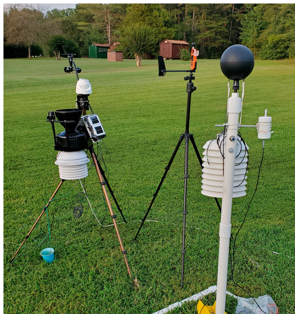
FIG. 1. Field work instruments (WBGT meters and weather station). The WBGT meter (right) with a black globe thermometer, natural wet bulb temperature probe situated in a water reservoir, and dry bulb sensor in a radiation shield. A weather station (left) and a Kestrel 5400 (middle) were also collocated with the WBGT meter.
