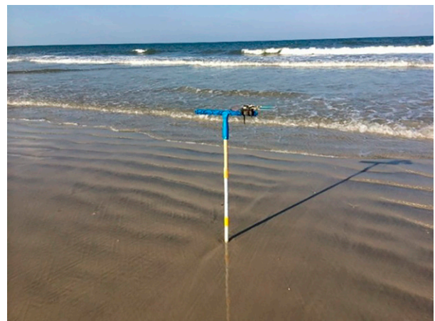
FIG. 9. Continuous wave radar setup at Mickler Beach.
