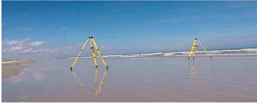
FIG. 12. Crescent Beach experimental setup with two tripod-mounted, first-generation radars.
