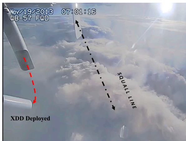
FIG. 16. Photo from the forward-looking, belly-mounted WB-57 camera documenting deployment of XDD (foreground left) at the beginning of a WB-57 sonde-deployment flight leg over the clouds associated with a squall line off the Texas coast (background right).
