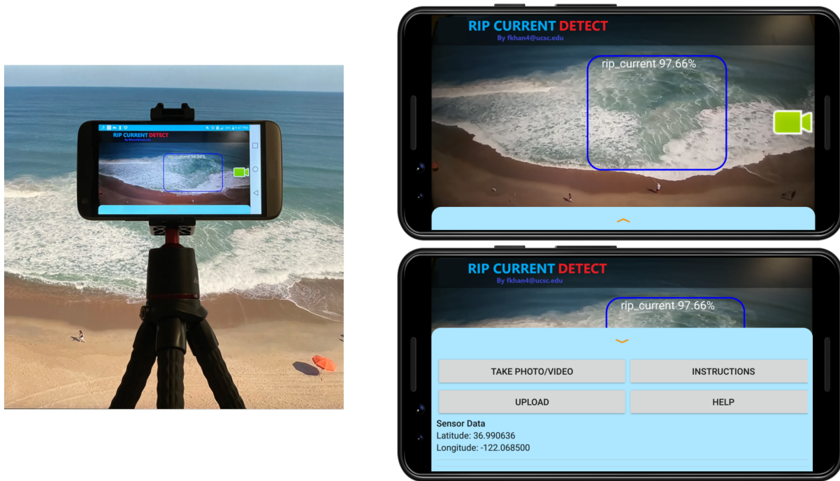
Figure 2: Left: app created by our citizen science platform in field work. Right: (top) detection bounding box with confidence score and (bottom) graphical user interface showing sensor information, data uploading and other options.
