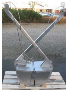
Figure 1. Van Veen Grab Sampler
