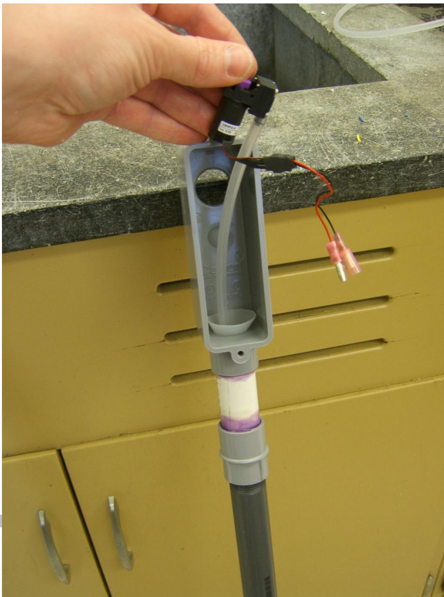
Figure S11 – Pump with splices crimped on, and flex-tubing cut to length. The tubing threads through a funnel inside the junction box, and the pump will sit in the funnel.
