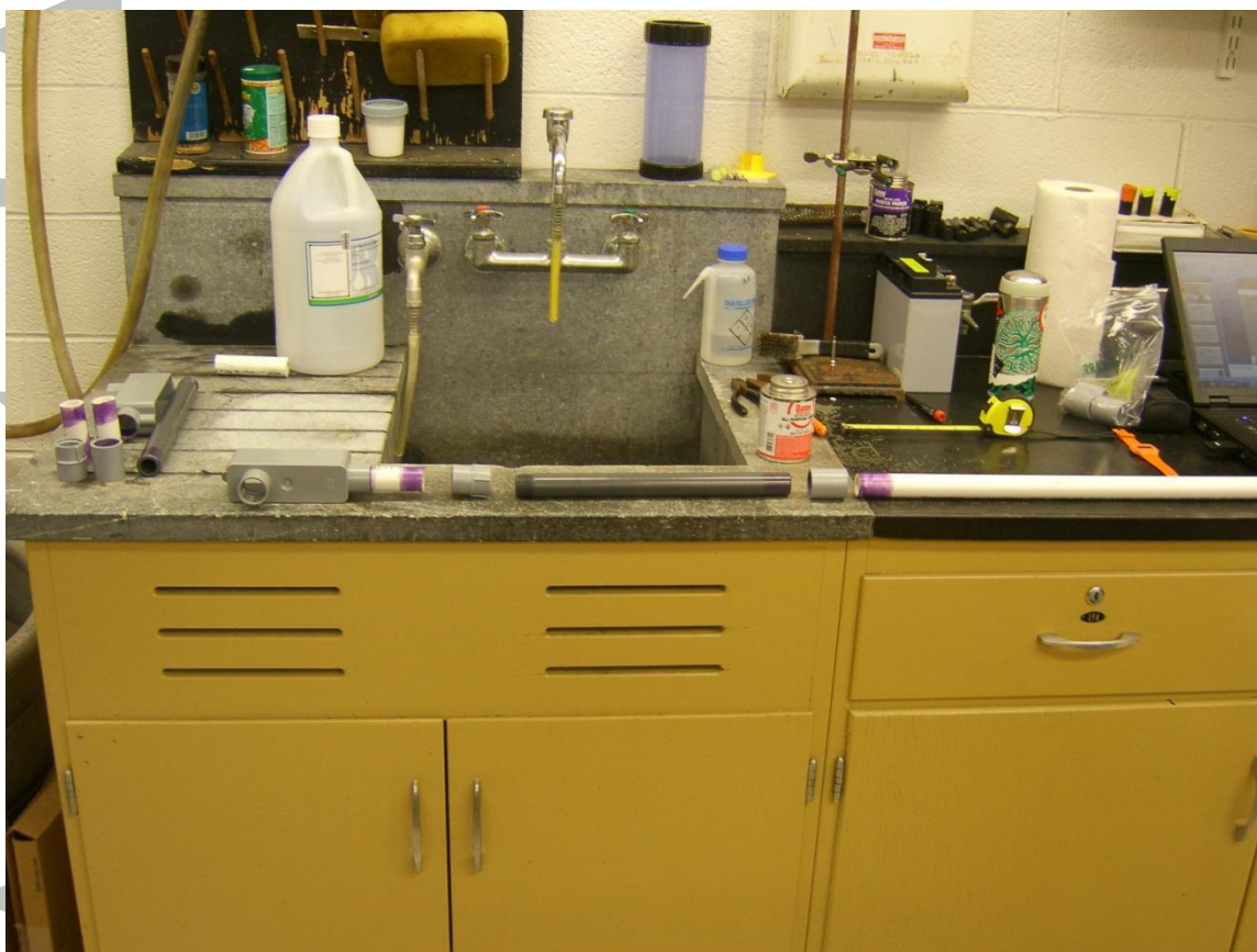
Figure S6 – Sections of housing prepped for cement
