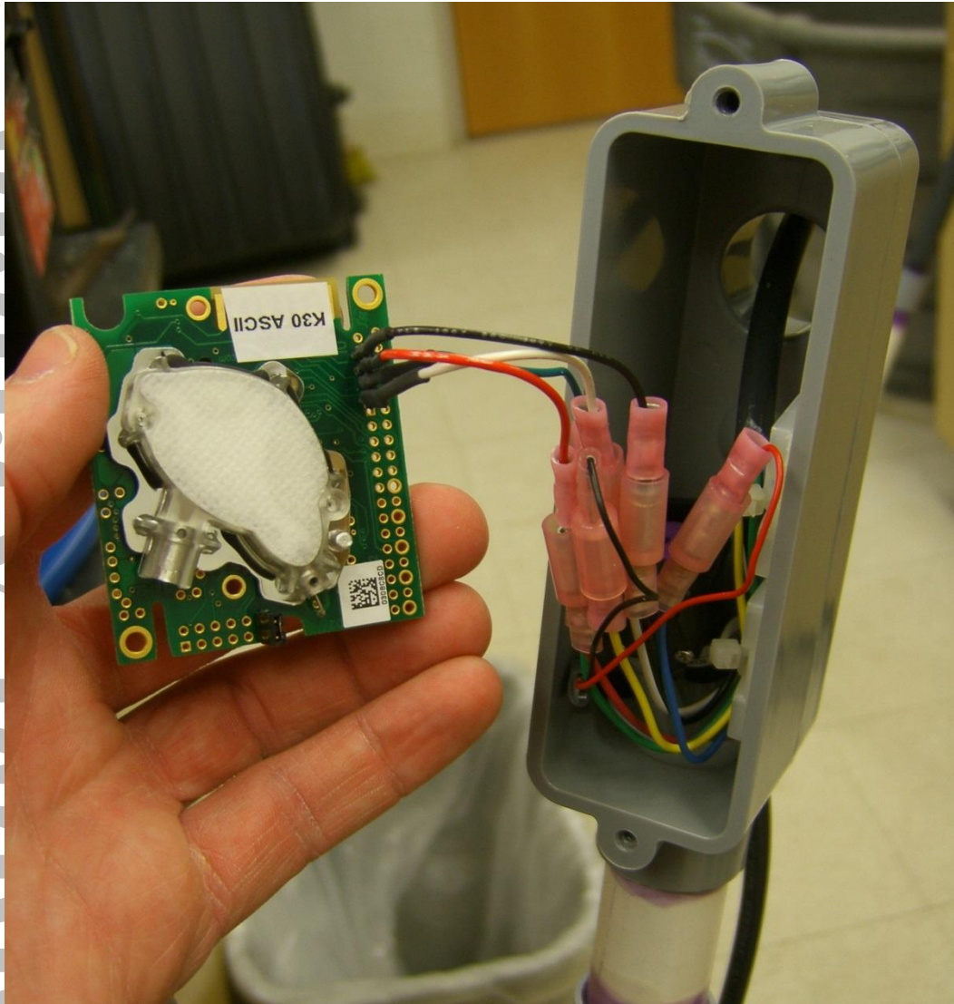
Figure S13 – Field Cable is connected to the CO 2 sensor and pump.
