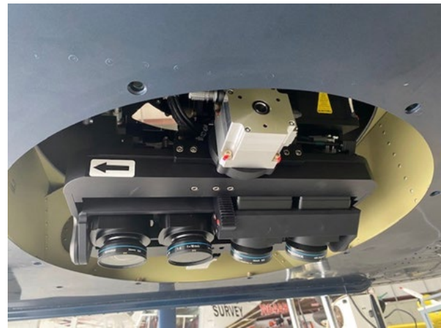
Figure 3: NOAA's System Aircraft Installation - The Multi-Camera System Component during Operation
