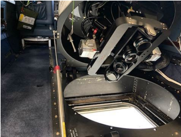
Figure 2: NOAA's System Aircraft Installation - The Multi-Camera System Component
