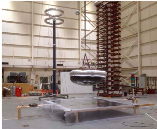
Figure 7. Setup for the second phase of the experiment at the high-voltage facility at Mississippi State University. The ambient E field between the upper negative and the lower ground electrodes in the 0.9 m wide gap is vertical; the particles were suspended on horizontal dielectric threads.
