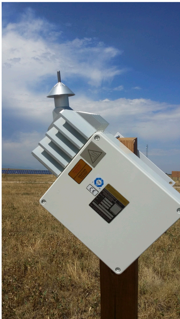
FIG. 2. Icing sensor used on the ASOS. The small, vertically pointing rod at the top is the actual probe that is used for detecting icing conditions.
