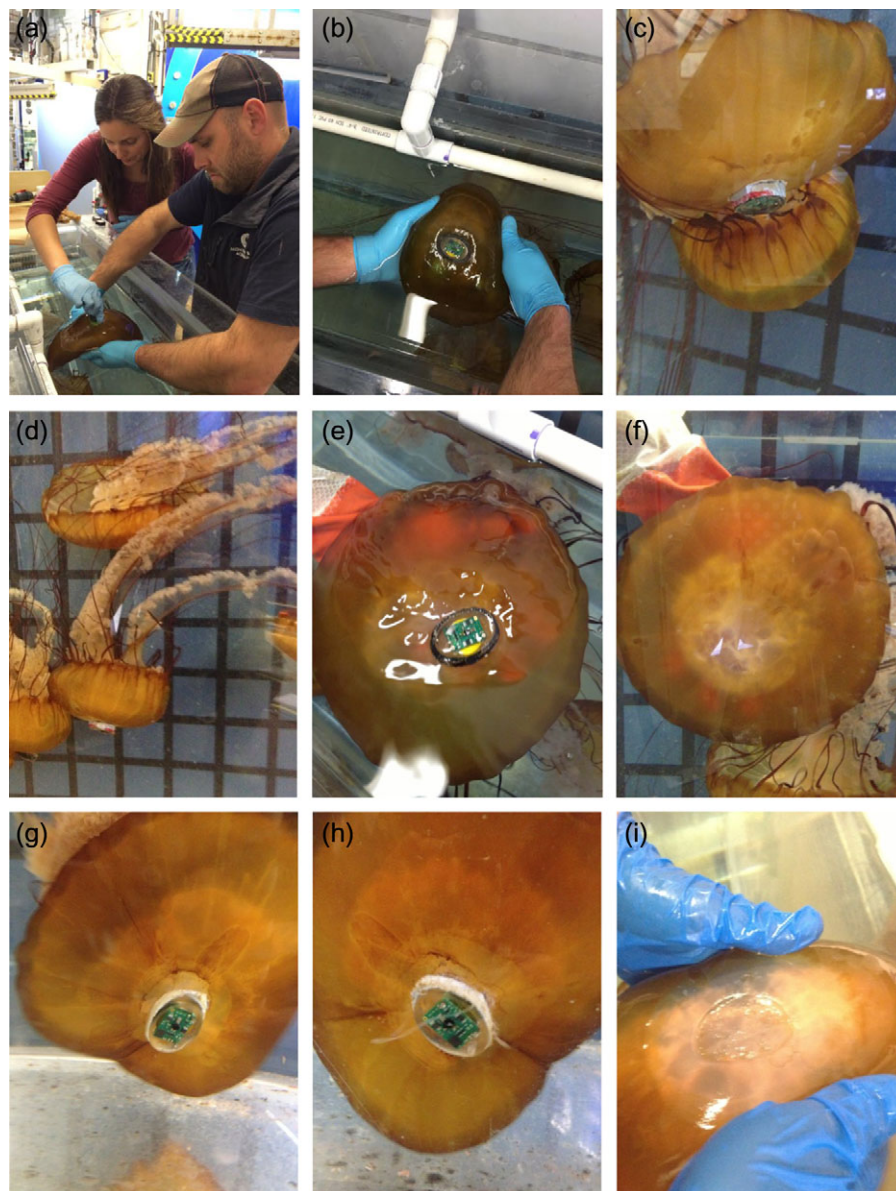
Fig. 2. Deployment of a tri-axial accelerometer on two Pacific sea nettle jellyfish Chrysaora fuscescens using the “glue” method. (a–f) Photos of a first individual on day 0 (a, b), day 6 (c), day 13 (d), day 22 (e), day 22 after tag was retrieved (f). A slight discoloration of the bell and around the logger’s previous location is apparent. (g–i) Photos of a second individual equipped on day 23 (g), day 27 (h), day 27 after logger fell (i). In this case, a discoloration and superficial peeling of the jellyfish bell were apparent.
