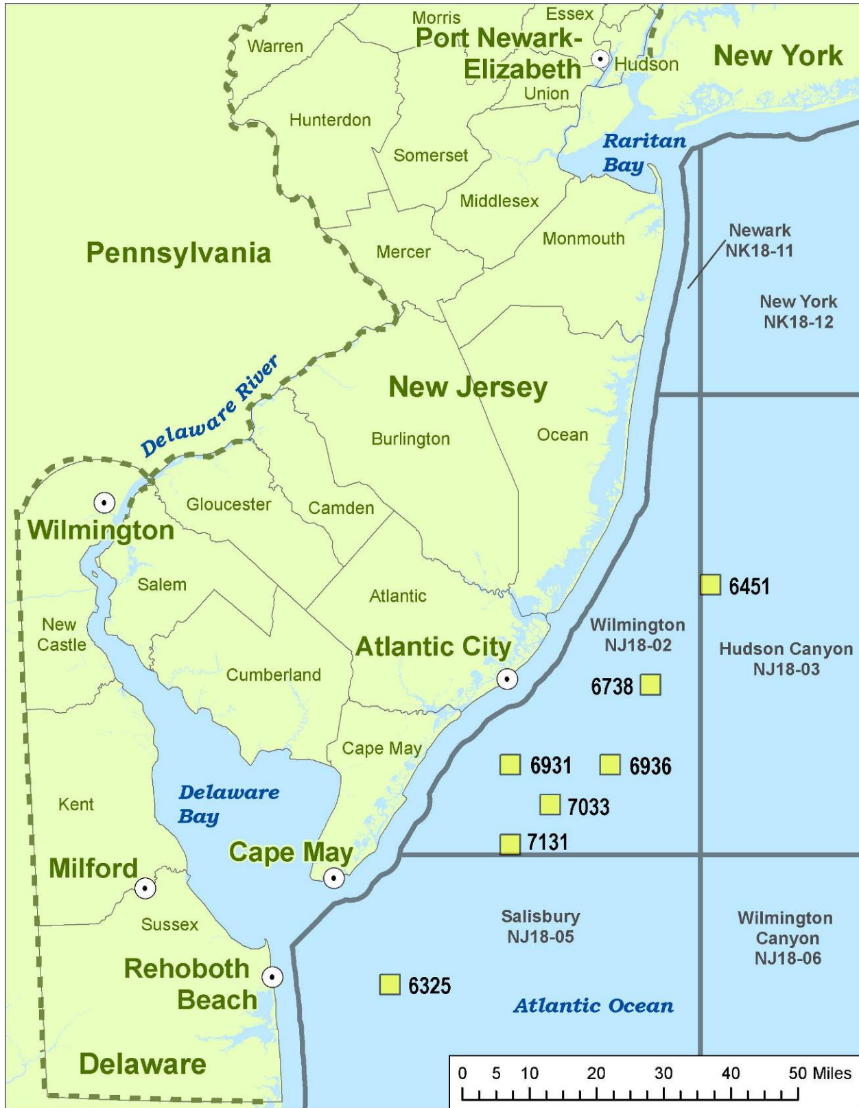
Figure 1-1. OCS blocks proposed for wind resources data collection off of Delaware and New Jersey.
