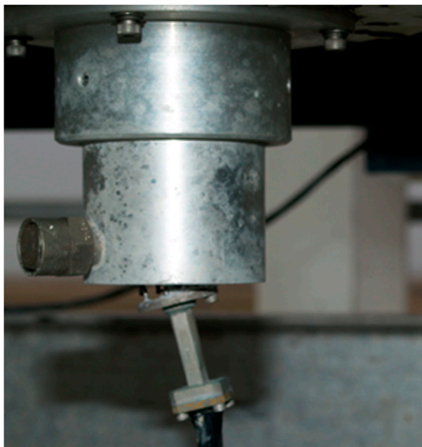
FIG. 17-4. The waveguide from the NSA MMCR has worked its way free from its connection to the antenna port. This was a slow process that spanned many months of the harsh Arctic environment at the NSA site.
