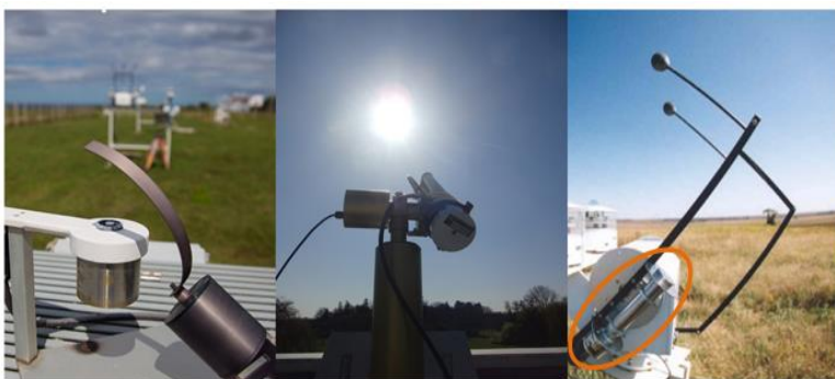
Figure 1. Images of three ground-based instruments for measuring AOD at the ARM SGP CF: MFRSR (left), CSPHOT (center) and NIMFR (right).
